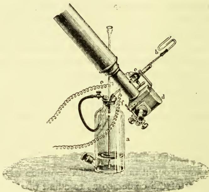
Huggins' Apparatus for observing the Spectra of Hydrocarbons.
