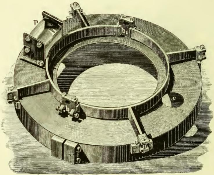
Merz's Object-glass Spectroscope. (Mounting of the Prism.)
