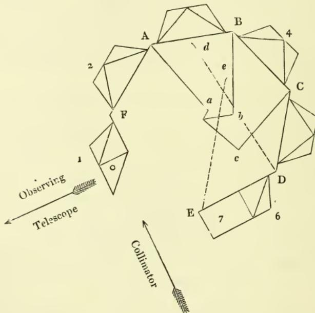
and are finally received, emerging from the first fixed semi-prism, by the right-angled prism of total reflection 8, and so passed to the observing telescope, which is placed at right angles to the collimator merely as a matter of preference. Any other position can be utilized if desired.
