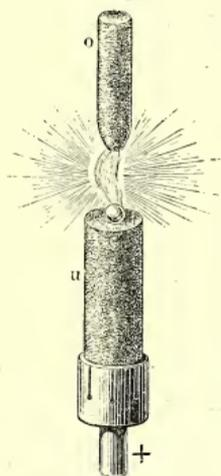
Volatilization of Metals in the Electric Light.
