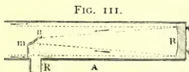
Path of the Rays through the Telescope.
