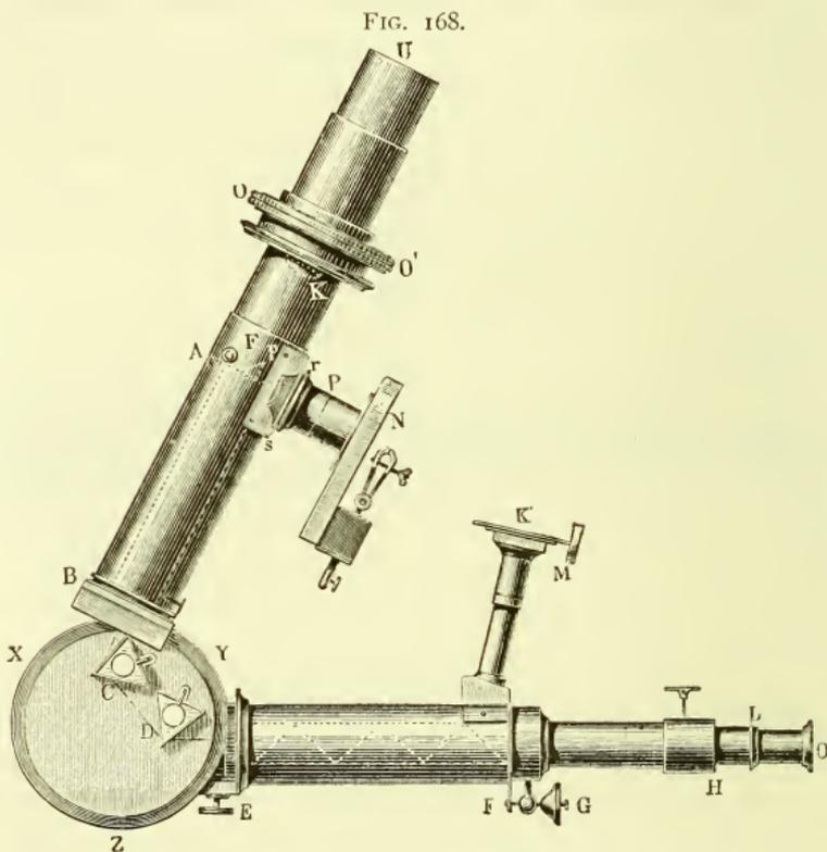
Secchi's large Telespectroscope.
