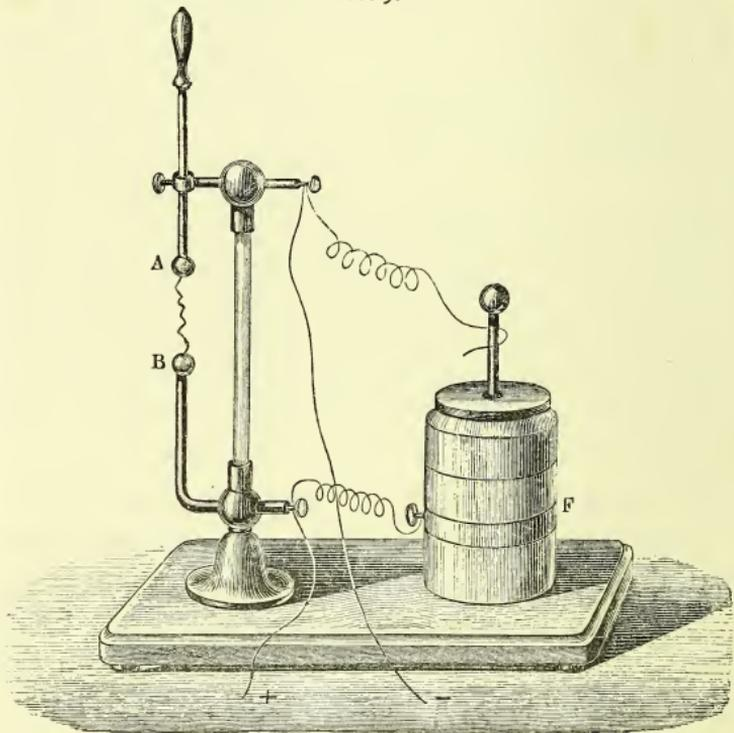
The Electric Spark intensified by a Condenser.
