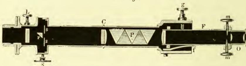
Merz's simple and compound Spectroscope.
