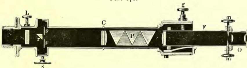
Merz's Simple and Compound Spectroscope.
