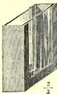
Glass Vessel for Absorbent Liquids.
