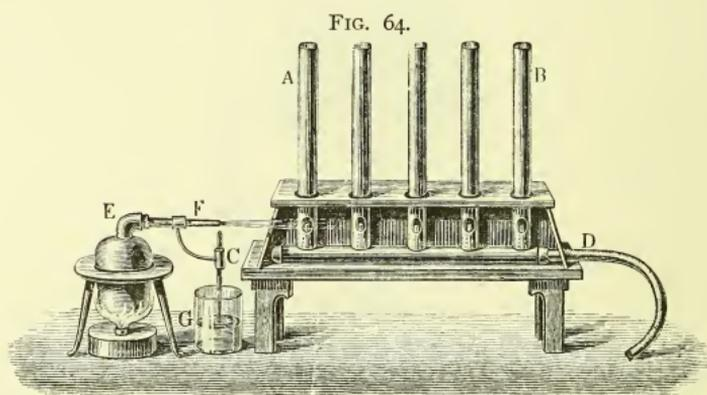
Morton's Apparatus for Monochromatic Light.
