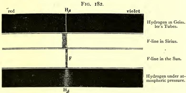
Displacement of the F-line in the Spectrum of Sirius.
