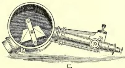
of the slit. The parallel rays emerging from the lens *g* pass through two dense flint-glass prisms *h*, *h*<sub>1</sub>, possessing a refracting angle of 60°, by which they are decomposed, and a spectrum formed which is examined by means of the small achromatic telescope *p*. In order to measure the distances between the lines of the spectrum, the telescope can be turned upon a pivot by means of a fine micrometer screw *q y*.
