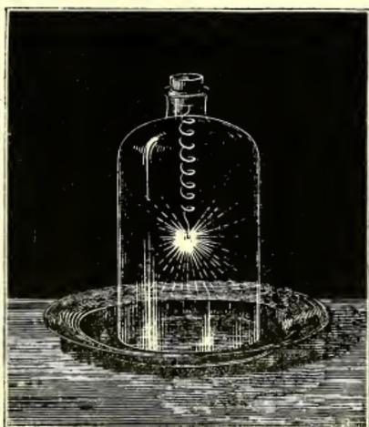
Combustion of a Steel Watch-spring in Oxygen.
